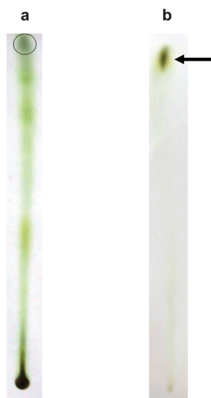
TLC purified compound of MeOH extract of C. Quadrangularis . Mobile phase 1:9 ratio of Hexane and Ethyl acetate. a) Separation of Crude extract compounds b) Partially purified compound, unlabelled arrow showed the single spot.
